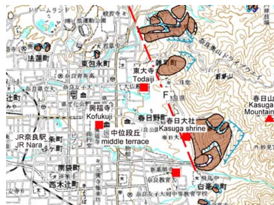
Figure 12 Distribution of slope failure topography near the Nara Park. Courtesy the National Research Institute for Earth Science and Disaster Prevention website.
