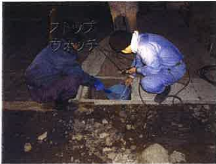
Measurements of drawn water (Pumping water up at a rate of 40 litter/min)
