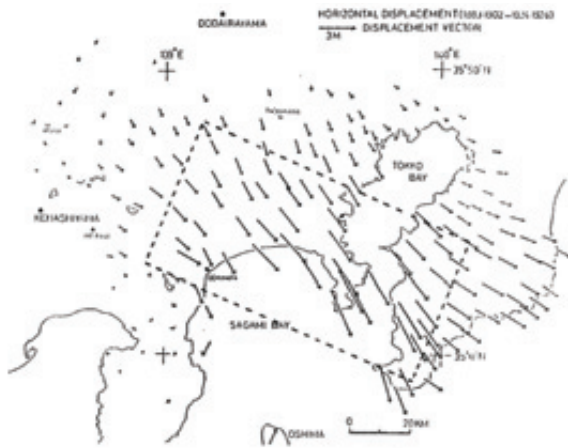
Fig. 2. Horizontal displacement vector caused by the Kanto earthquake derived from the second order triangulation stations (NAKANE [4]). A fault plane projection obtained by MATSU'URA [7] et al. is drawn by a dotted line.
