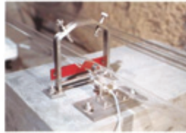
伸縮計の中間センサー An in-between part sensor of an extensometer
